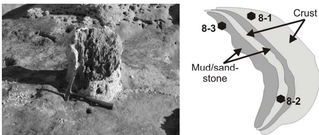
Fig. 6: A small piece of the chimney (shown on the left) was sampled for laboratory analyses (sample 8). The scheme to the right shows the sub-sampling strategy
